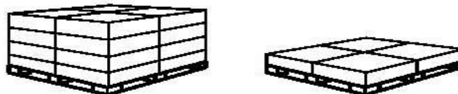
Properly Palletized Unit Load (Leveled Layers)
